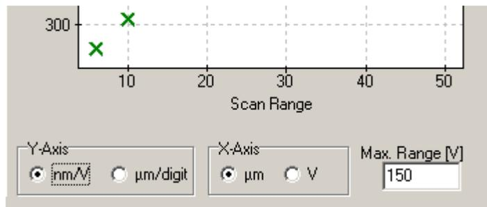
Chose the tick “nm/V” instead of “µm/digit”, and the entries I the scan range table are recalculated in nm/V and displayed in this unit.
