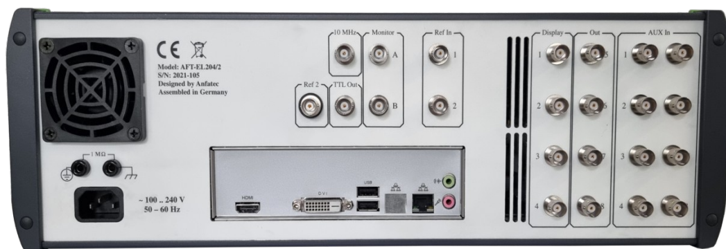
Figure 9: Rear-Panel of the eLockIn (picture might vary from current revisions). The ground connector above the power supply allows to separate the protective ground from the housing and thus increase the resistance between them to 1 MOhm.
